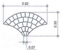
ANGULAR DESIGN OF CONCRETE STAMPED
