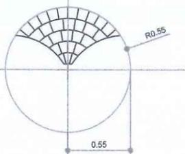
reference point to get the radius of the concrete stamped.
