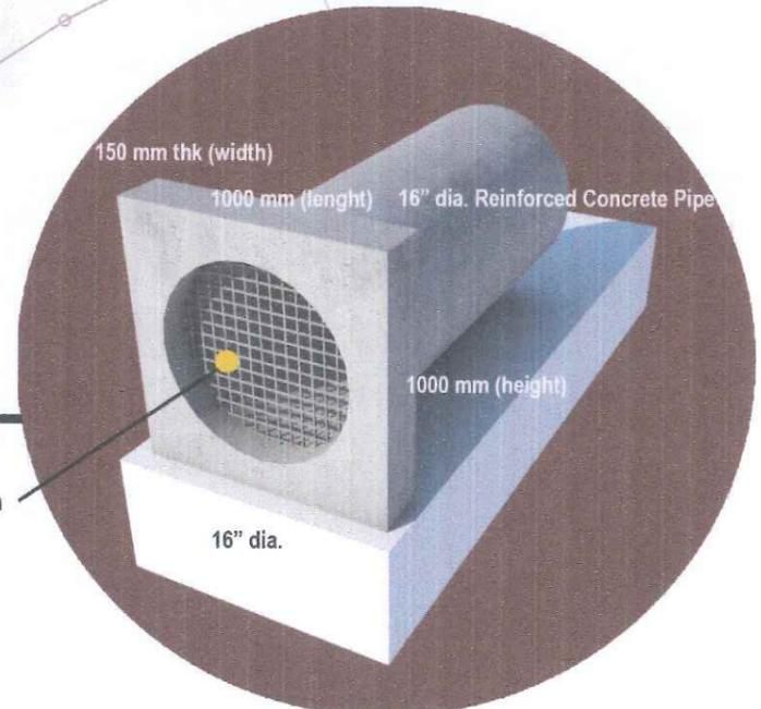
14 -10 mm DIA. DEFORMED BAR- bothways with a 50 mm space between deformed bars .
