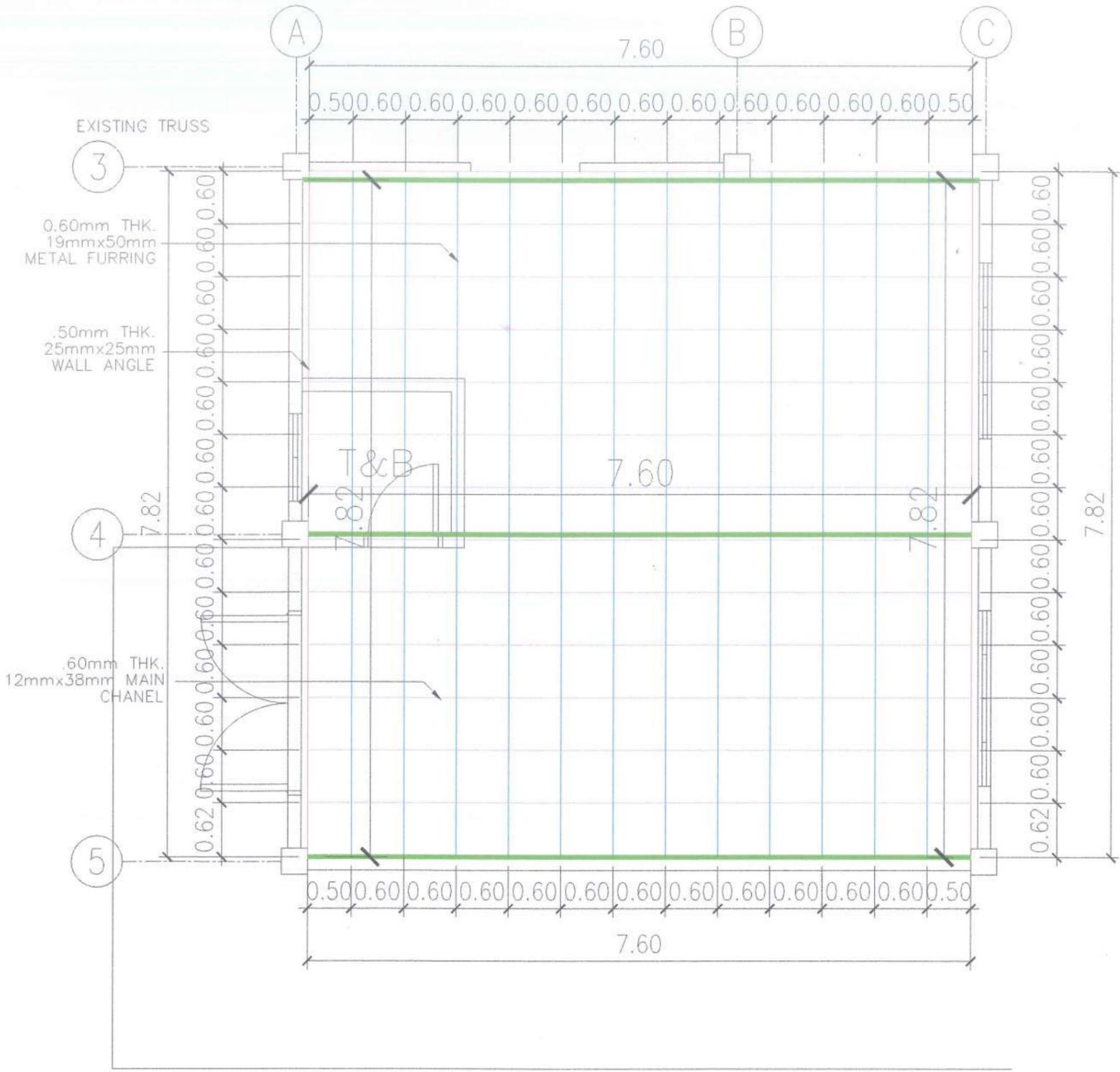
**2 CEILING FRAMING PLAN BLOW-UP PLAN**
